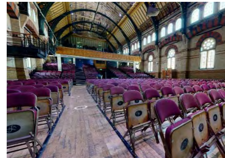
Inset gangways occupy prime, optimum sightline positions where there should be seats (whilst the seats are pushed to the perimeter).
