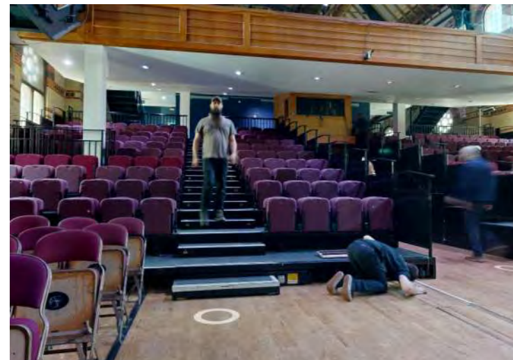
With its convoluted arrangement wrapping around the columns, the retractable unit is more complex to operate, extending turnaround times.
