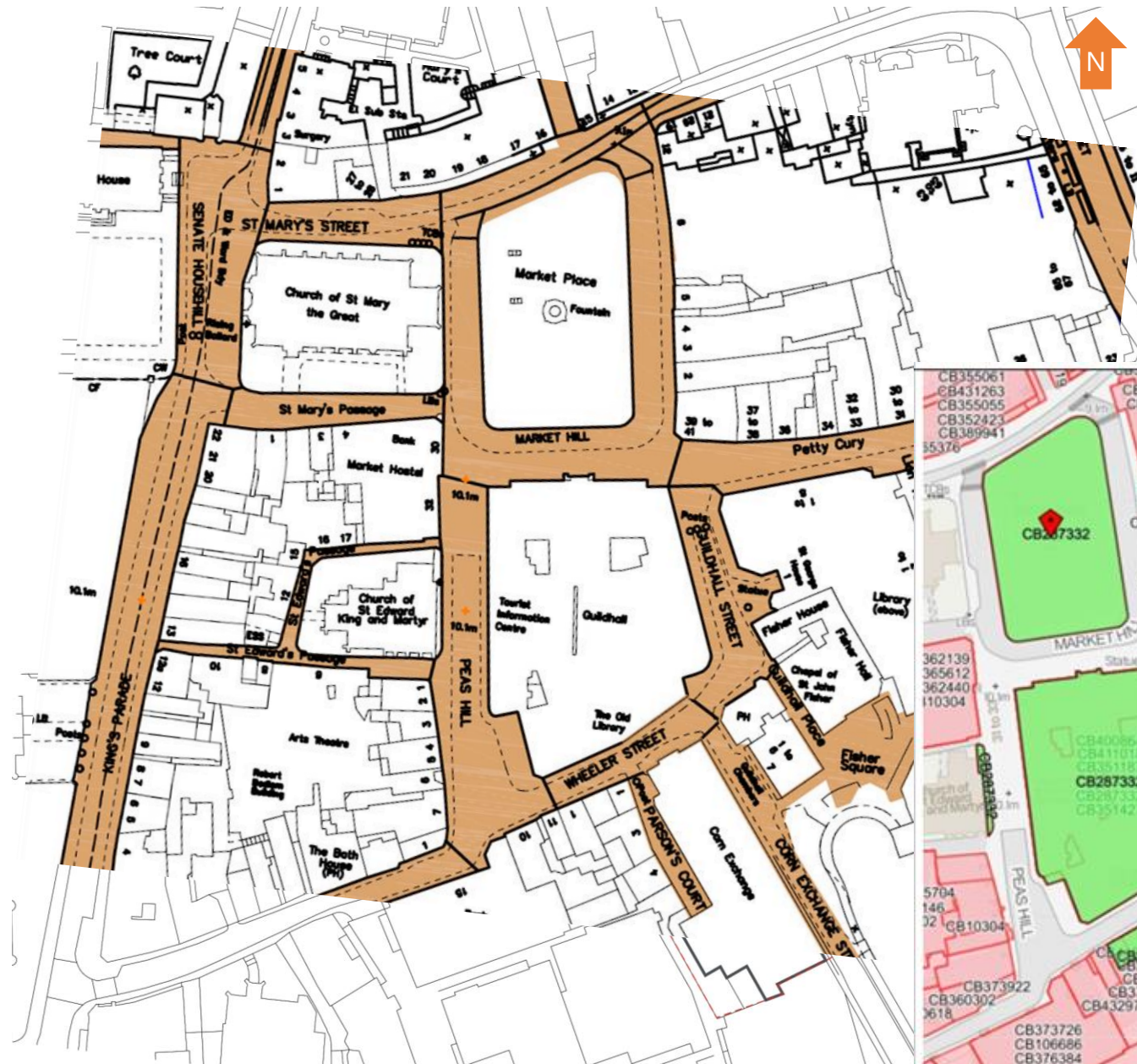
Fig. 4. Indicative Highway Boundary Data
