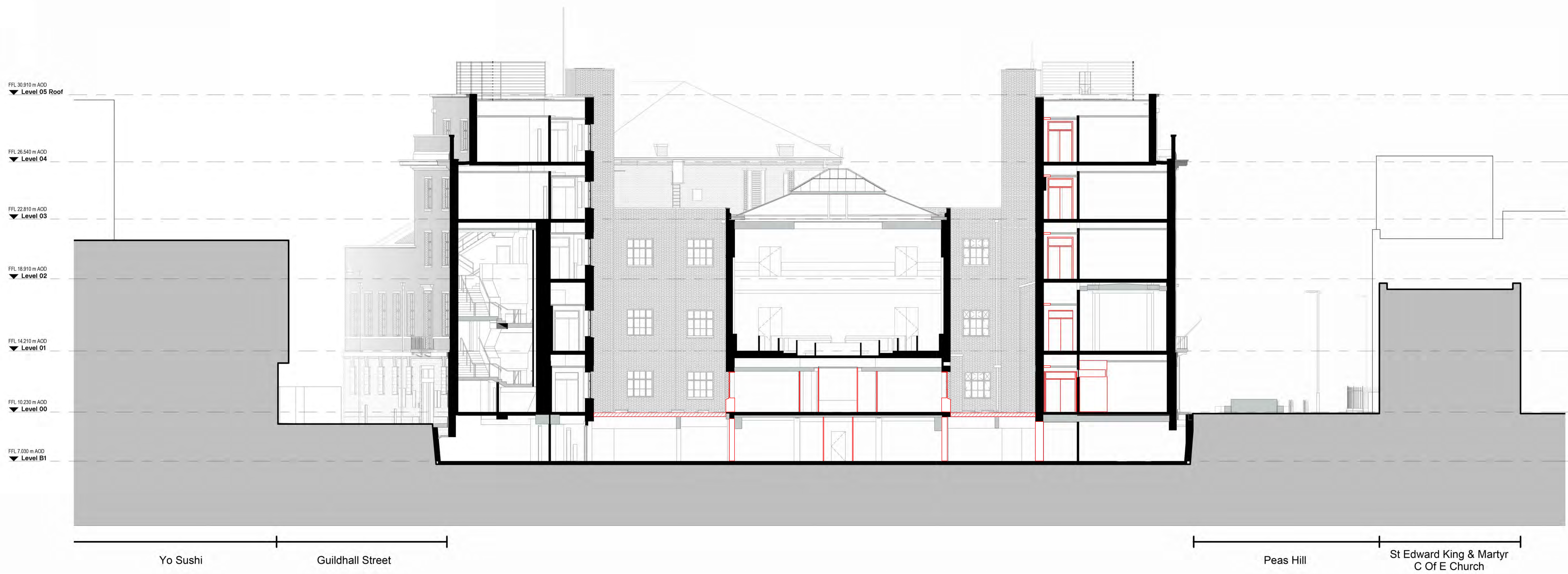
Existing Section AA with Proposed Demolitions 1:100
