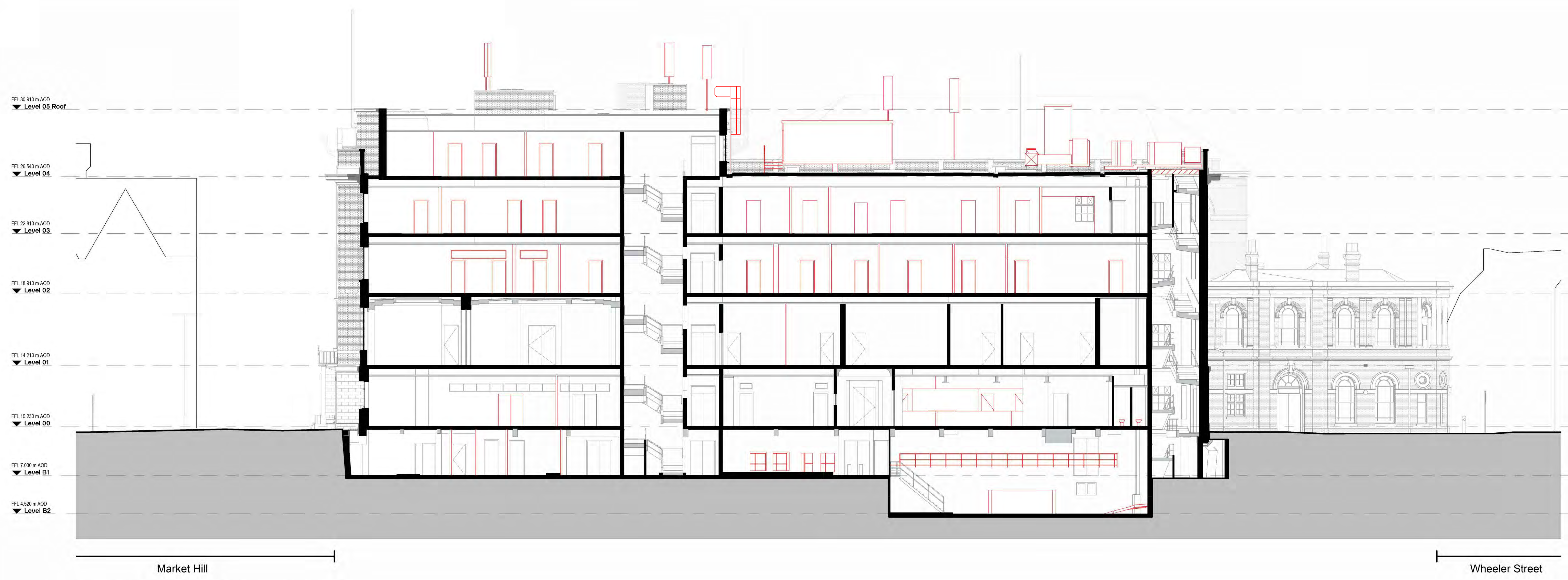
Existing Section BB with Proposed Demolitions 1 : 100
