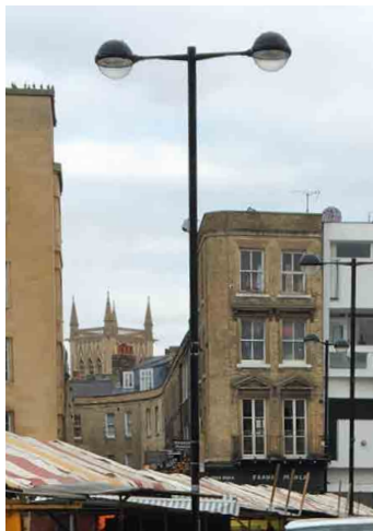
Double lighting posts DW Polar 500 Lantern 140W CPO-TW Lamp 8m high- RAL 9005 (Jet Black)
