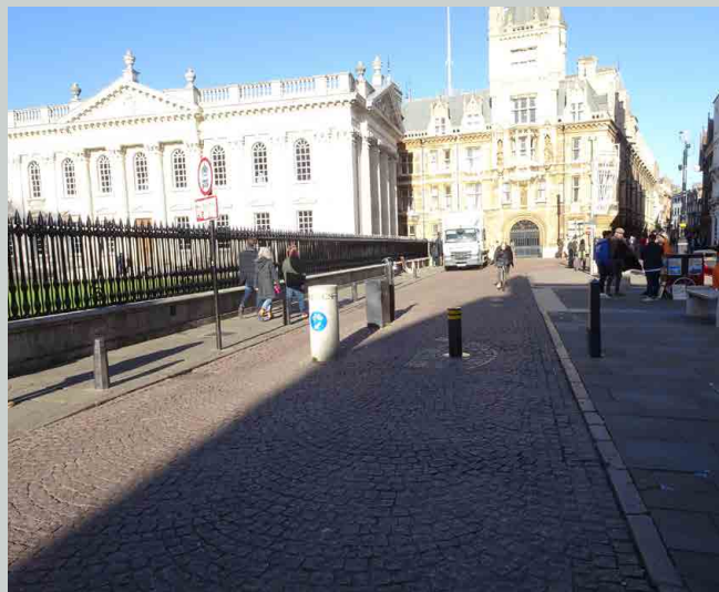
Rising and fixed bollards on Senate House Hill at the junction with King's Parade
