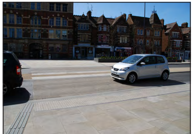
Figure 29: Courtesy pedestrian crossings replace the old signal controlled crossings. The 8m width of the crossings respond to key desire lines and simplifies the pedestrian experience (Frideswide Square, Oxford).
