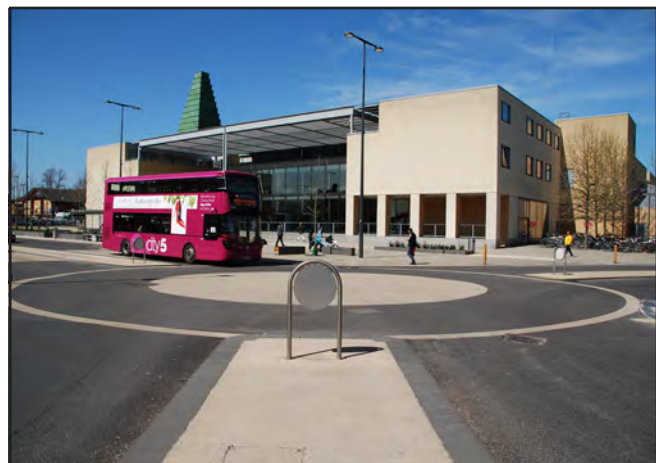
Figure 34: Roundals creates a series of distinct spaces. Median strip (2.5m) separates the direction of vehicle movements, tightens approaches to junctions and provides for informal crossings. Limited signage and road markings encourages lower vehicle speeds (12-15 mph) and assists traffic flows. (Frideswide Square, Oxford).
