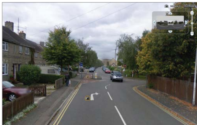
Figure 60: The existing situation... Uninterrupted views, wide carriageway widths and narrow footways, reinforce vehicle dominance. (View looking west along New Street towards Harvest Way junction)
