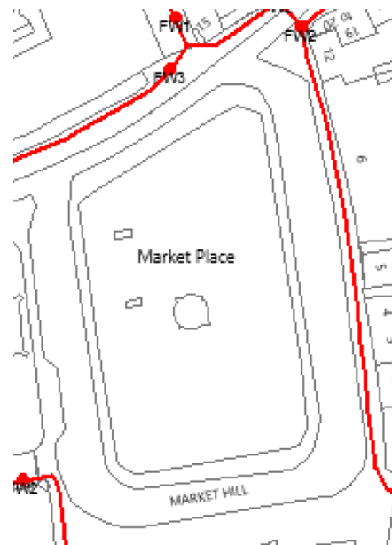
The above extract shows that there are no existing Virgin Media services routing into the Market Square. There is existing infrastructure on the far (north) side of St Mary's Street and east (retail/shop) side of Market Hill. A service also emanates from Peas Hill and is shown turning and terminating in the junction to St Mary's Passage.
