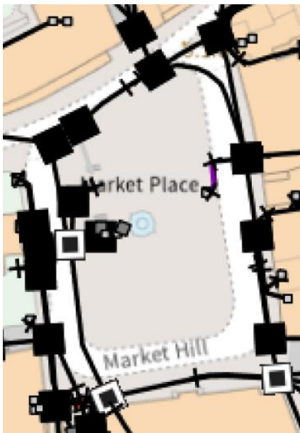
The above extract from the BT Openreach utility map shows the existing BT infrastructure located around the north, east and west sides of the Market Square, however, there are no direct connections to any stalls. The filled in black area represents a 'box' and the white concentric squares represent a manhole.
