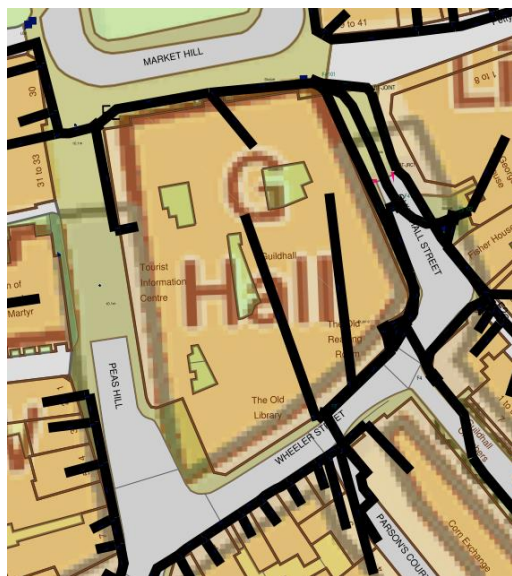
The Cityfibre drawing extract above shows possibly four telecommunication points entering the building with two of these routing through the Sticks'n'Sushi demise.
