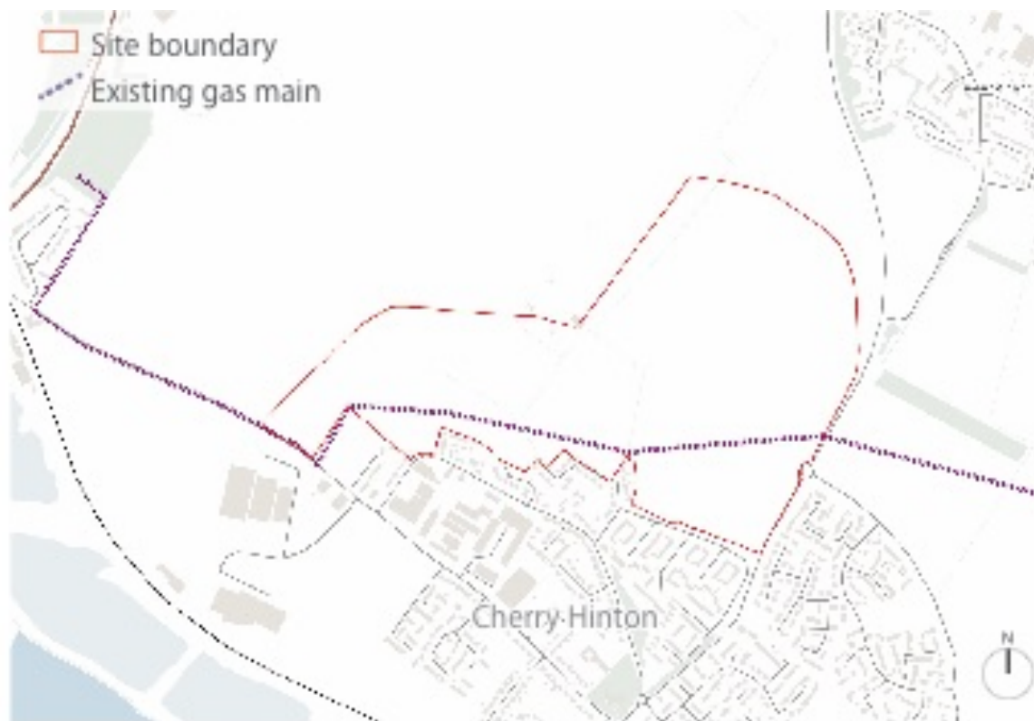
Figure 34: Existing gas main
