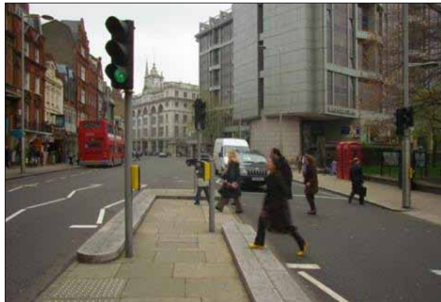
Figure 73 - Crossings have been redesigned with the removal of guardrails (Kensington High Street, London)
