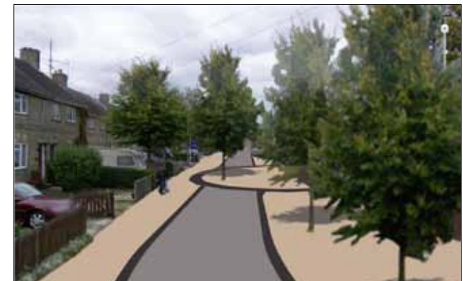
Figure 85: A possible solution? Placemaking at intersections - circular design at junction with Harvest Way celebrates the allotments and existing 'pocket park'. Trees located within the 'apparent' highway frame the space and encourage drivers to slow down. (Artist impression of Project 5: proposed improvements along New Street/Harvest Way)
