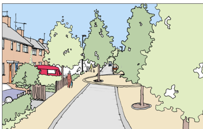
Figure 63: A possible solution? Placemaking at intersections - circular design at junction with Harvest Way celebrates the allotments and existing 'pocket park'. Trees located within the 'apparent' highway frame the space and encourage drivers to slow down. (Artist's impression of Project 5: proposed improvements along New Street/Harvest Way looking west)
