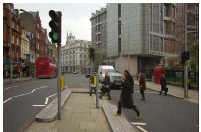
Figure 53: Crossings have been redesigned with the removal of guardrails (Kensington High Street, London)
