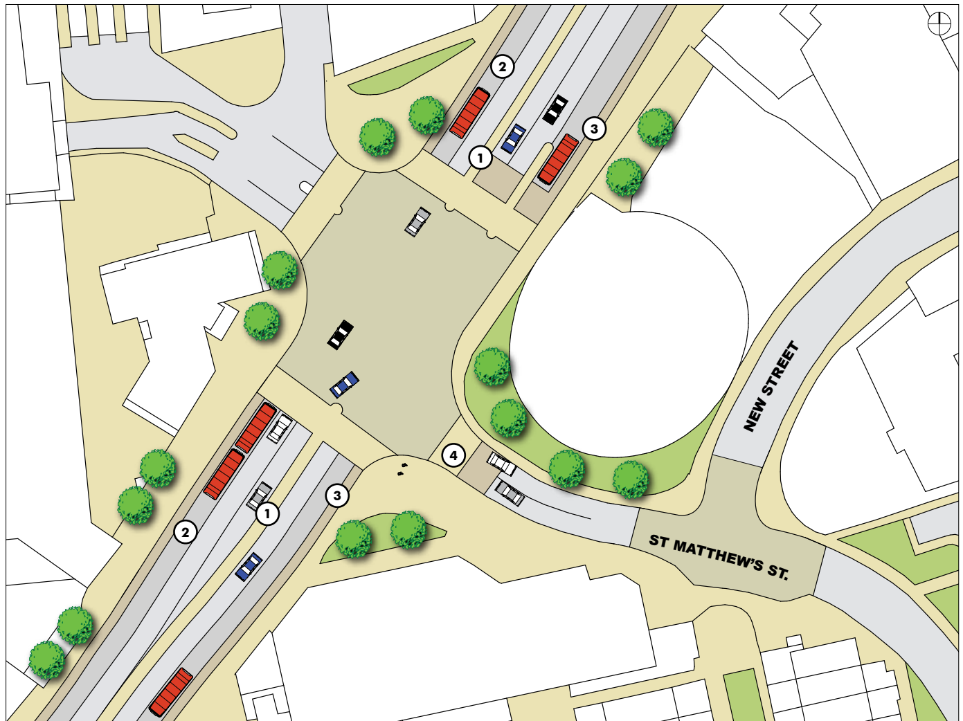
Figure 56: Key Project 3 - Illustrative proposal for the remodelling of St Matthew's Street Junction
